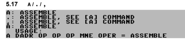
Assemble, the entered mnemonics and parameters will be translated to machine code and stored in the memory. (All three commands perform the same function.) If the illegal codes option is enabled, those can also be entered. Unlike in the **TEDMON**, even the disassembled code column (produced with the "**D**" command) can be modified - with certain restrictions. (For example, changing the address of a parameter will update the address of the memory.)
